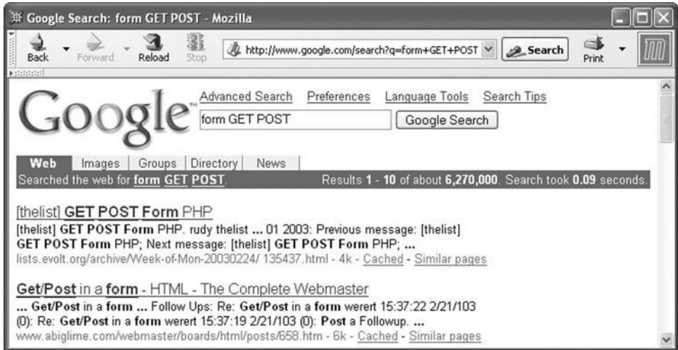
FIGURE 6.10 Example of search page generated by a form using an HTTP GET method. The Location bar shows the URL (with some parameters removed for simplicity) generated by the form. (This Web page is reproduced by permission of Google Inc.)
