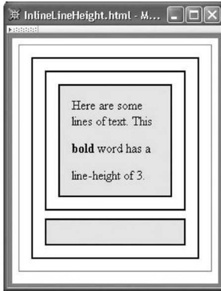
FIGURE 3.30 Effect of setting line-height on an inline element (the word “bold”).
