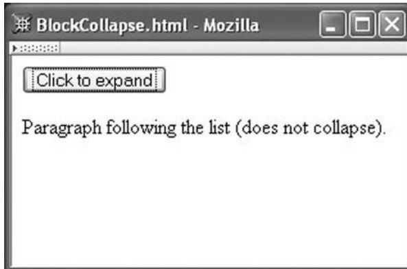
FIGURE 5.14 Rendering of BlockCollapse.html after button is clicked once (or any odd number of times).
