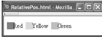
FIGURE 3.31 HTML document using relative positioning to nudge text to the left.
