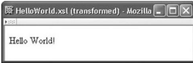
FIGURE 7.28 XML document containing an xml-stylesheet processing instruction that associates the XML document with an XSLT document.
