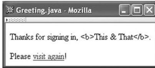
FIGURE 6.14 Thank-you page of the Greeting servlet. The user signed in as <b>This & That</b> ; notice that the XML special characters are displayed rather than being treated as markup.
